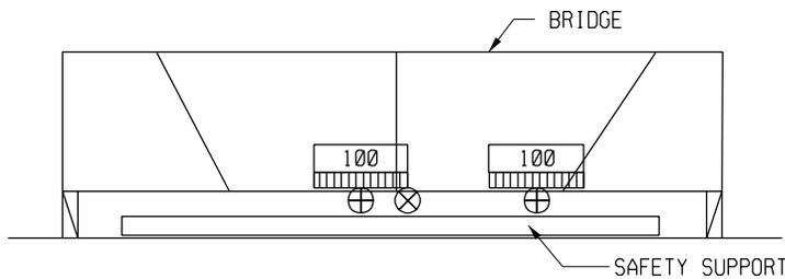
**0** VERTICAL LOAD TEST - PRELOAD
