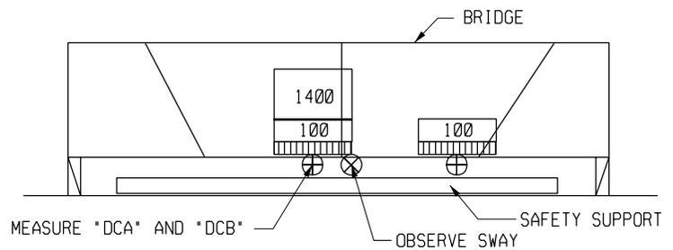
**1** VERTICAL LOAD TEST - STEP 1
