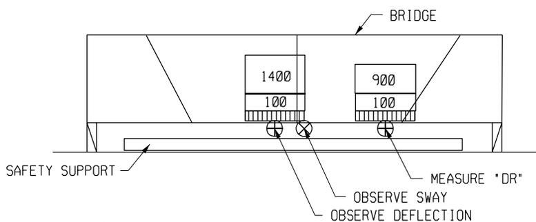
**2** VERTICAL LOAD TEST - STEP 2
